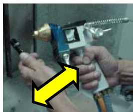
Strike a spark at the air cap outlet,
