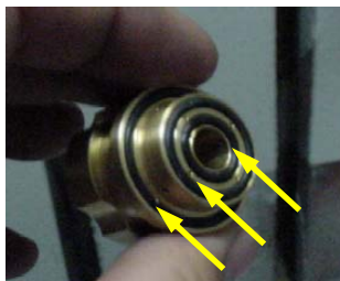
Insert 5x O-rings. Use specific O-rings supplied by SG-SNMI. Each O-ring is different: the 2 mat color O-ring must be on the front.
