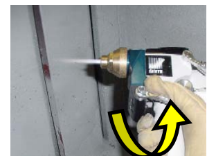
Turn the gas valve gradually and smoothly to position 3 "Full gas" and start the wire,
