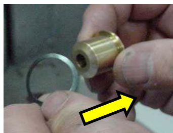
▲ Insert the ring on the air cap
