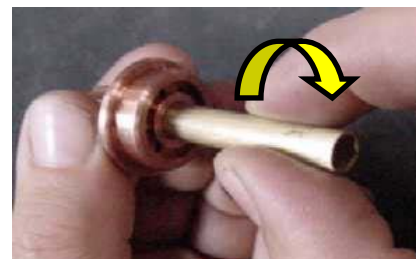
▲ Insert and screw the wire guide tube
