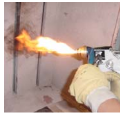
Ignition of the gun (over 3sec air cap could be damaged)
