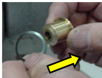
▲ Insert the ring on the air cap
