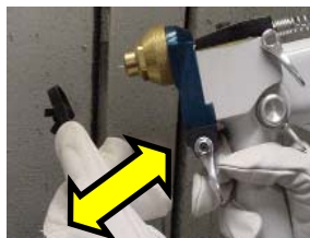
Strike a spark at the air cap outlet,
