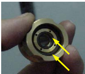
Insert 5x O-rings. Use specific O-rings supplied by SG-SNMI. Each O-ring is different: the 2 mat color O-ring must be on the front.
