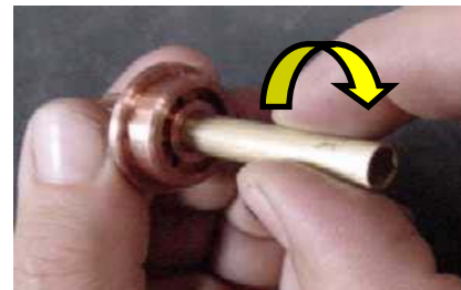
▲ Insert and screw the wire guide tube
