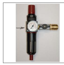
Mount included air service unit for air motor and connect it in vertical position with air supply.
