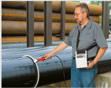
Porosity detection on pipelines
